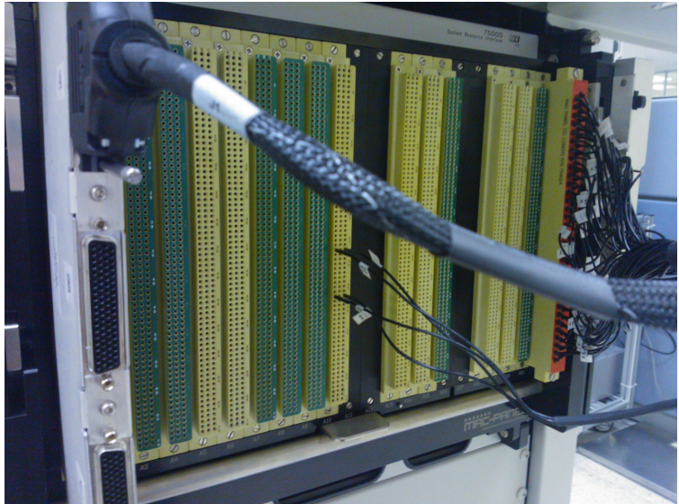
Figure 3-6 Installing a Universal CEDGN Test Fixture U8972-67901 with a CEDGN HD Load Card Cable U8972-61629
