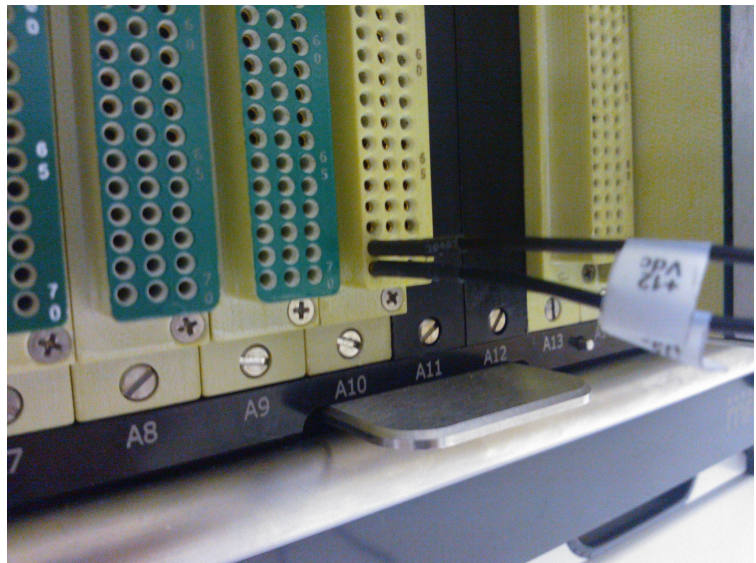
Figure 3-8 The Power Pins of the CEDGN E-Load Cable U8972-61630 are manually probed to ICA Slot 10
