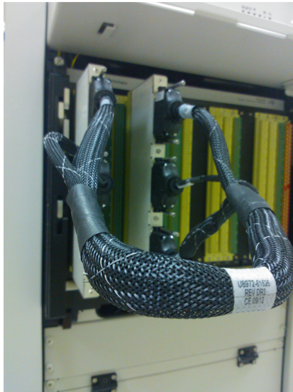
Figure 3-9 Installing two Universal CEDGN Test Fixtures U8972-67901 with a CEDGN HV-DAQ Cable U8972-61626
