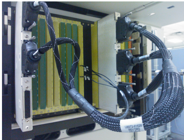
Figure 3-4 Installing two Universal CEDGN Test Fixtures U8972-67901 with a CEDGN Load Card Cable U8972-61628
