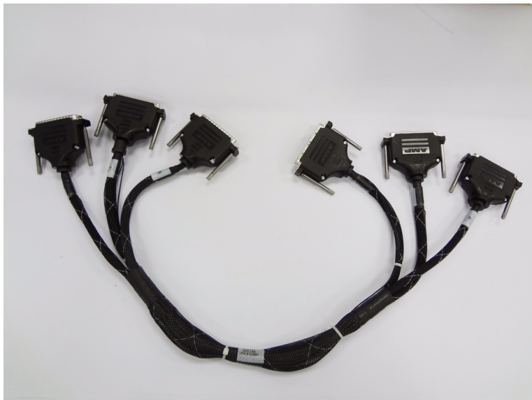
Figure 4-53 CEDGN Cable (U8972-61627 CEDGN SYSTEM UTILITY CABLE) for System Utility Test
